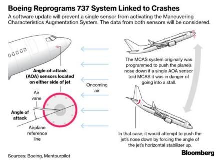
Boeing 737 Max was designed to react to only one of the plane's two "angle of attack" sensors that measure the jet's incline.
